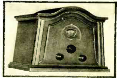
Above—Appearance of new Stewart-Warner short wave converter of the super-het type, supplied separately if desired; the same S-W converter, shown diagrammatically at the left, is also “built in” on the new Stewart-Warner console for broadcast reception.
