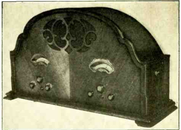
Above: The new Pilot "All-Wave" super-het with "wave change" switch. Range 10 to 550 meters.
